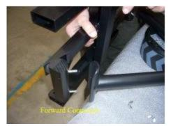
Starting by guiding the Forward Connector into position so the two threaded studs fit into the holes in the CORE trainer leg.
