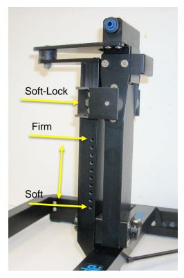
Tilting Force is controlled by the height of the Spring Mounts on the side of the Fork Stand. There is a soft-lock position and 8 softer settings ranging from High (Firm) to Low (Soft).
