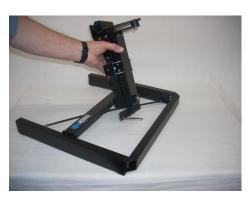
Carefully attach the Fork Stand to the forward side of the base by inserting all 8 screws using the hex key. Do not fully tighten until all 8 screws are installed.
