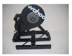
This is the finished rear assembly ready to be attached to the bike. Install the bike as you normally would, leaving front wheel on for now. Do not fully tighten the bike's rear axle until the fork stand is attached.
