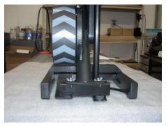
Now set the entire assembly upright. The Core should be sitting approximately vertical on the base. It should be free to rock side to side and move forward and back smoothly.
