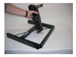
Carefully attach the Fork Stand to the forward side of the base by inserting all 8 screws using the hex key. Do not fully tighten until all 8 screws are installed.
