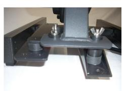
Once all three attachment points are loosely secured, hand tighten all three wing nuts.
