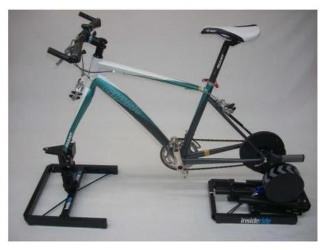
Photo shows Kickr installed. The basic configuration is the same for Kickr, Core or Hub trainers.
