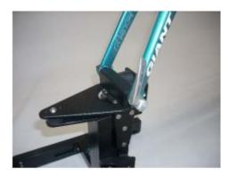
For Thru-Axle forks: Remove the blue inserts by pulling and twisting them out by hand or gently pull them out with pliers. They can also be pushed out using a QR skewer.
