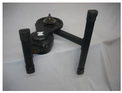
Lay the HUB on a table or countertop with the flywheel facing down. Hang the legs of the HUB over the table edge. Remove the two support bars from the HUB receivers.
