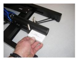
For proper forward positioning, the center leg of the KICKR should extend about 3" [76mm] from the front saddle.
