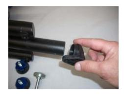
Prepare your KICKR for installation by unscrewing the 2 adjustable feet from the folding legs. Then remove the front foot from the center leg, that's held on with a single screw.
