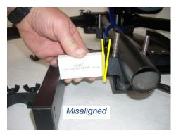
Use the Setup Block to check KICKR alignment. Slide the block between the Saddle Clamp and the frame as shown and check for visual alignment. If the saddle is out of square, rotate it back into alignment. Both front and rear saddle clamps should be checked.
