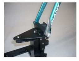
Lower the bike's fork onto the Fork Stand and tighten it with either the Quick Release or your Thru-Axle.
