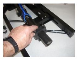
Install the 2 top Saddle Clamps, 4 wing nuts and tighten. The trainer should be approximately vertical and not heavily tilted to one side.
