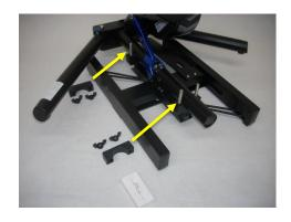
Lower the KICKR into position as shown. Place the center leg of the KICKR into the 2 Saddle Clamps on the E-Flex frame.
