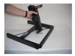
Carefully attach the Fork Stand to the forward side of the base by inserting all 8 screws using the hex key. Do not fully tighten until all 8 screws are installed.
