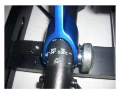
Next lower the Kickr height adjustment to the RD650C position and install the lock pin. The E-flex is designed to be used at this height position.
