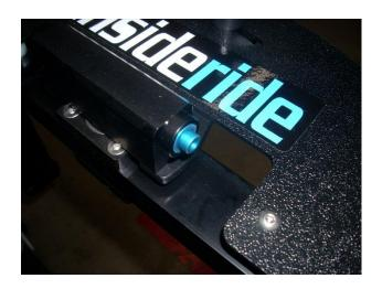
Point your fork straight ahead for proper alignment. Now tighten the rear dropout and you are ready to ride. Please read the user guide before riding. \*\*\*\*The E-flex does not alter the Kickr's resistance performance\*\*\*\*
