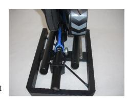
install the bike onto the Kickr. Use the normal Kickr installation procedure for attaching the bike. Leave your front wheel on for now.
