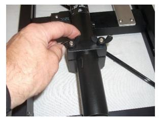
Install the 2 saddle clamps and 4 wing nuts and tighten by hand only.
