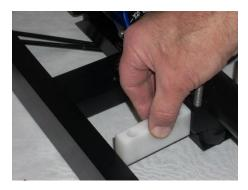
Use the provided setup block to check KICKR alignment. Slide the block between the saddle clamp and the frame as shown. First at the front clamp and then at the rear clamp. Adjust the KICKR position until the setup block just fits at both points. That will ensure the KICKR is aligned with the E-FLEX frame
