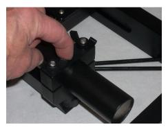
Install the 2 saddle clamps and 4 wing nuts and tighten. The trainer should be approximately vertical and not heavily tilted to one side. It does not need to be perfectly vertical to work properly. If it is tilted more than a degree or two, you may need to go back and adjust the support arm.
