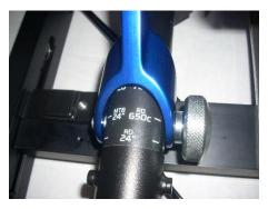
Next lower the KICKR height adjustment to the RD650C position and install the lock pin. This setting works for all KICKR models except the KICKR 20 (V5) which uses the RD 24 position to maintain a level ride height.
