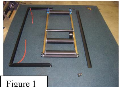
Unbolt and remove both the front and rear bumpers. You may need to use the thin wrench (supplied with the new belts) to hold the axles from turning while the bolts are loosened. (Figure 2)
